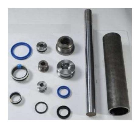
Honed Tube and Chrome Plated Shaft Cut Cutting Piston, Rear Cover, Front Cover Materials Preparation of Sealing Kits
